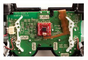
B. Once in fold the Flexboard Down on to the motherboard.
